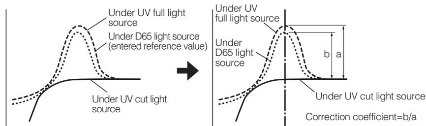
These correction coefficients are then used to obtain the fluorescent reflectance by performing numeric calculations using the measured reflectances under the UV full light source and under the UV cut light source. (The reflectances at cut wavelengths under UV cut light source are set to 0%.)
