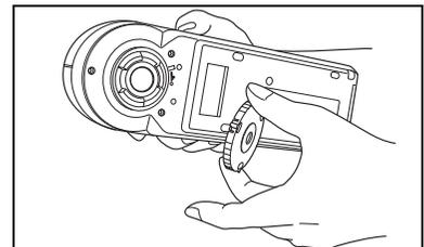
3. Use a blower to remove dirt and dust from the integrating sphere.
