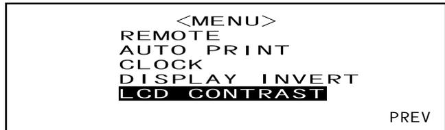
The contents displayed on the LCD will be reversed each time
