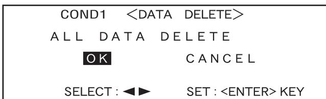
During global deletion, the amount of deleted measured data will be displayed in a percentage.
