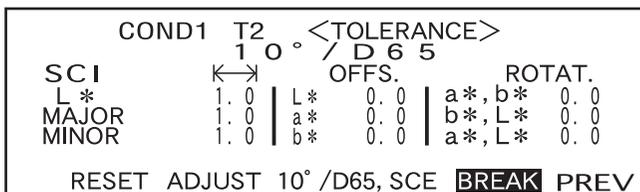
**6** Place the specimen measuring port to the specimen, and then press
