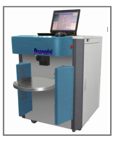
Power:220V/50Hz/3A,110V/60Hz/6A Number of canisters: 16 or 24 Volume of canister: 2L Compatibility: water base or universal colorants Max flow rate: 0.2L/min Precision:+-1% Minimum dispense quantity: 0,03ml Dispense type: sequential dispense Pump type: cavity bolts pump Capping system: automatic humidifier cap Nozzle size: diameter 2.5mm
